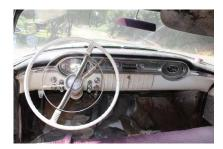
The driver's seat is covered by a black seat cover that has bleached out to a purple color via sun exposure. Beneath the cover, the seat material is a worn, but the seat isn't sagging. Dampness has worked away at the cloth and there are mild surface rust areas on the metal dash.
